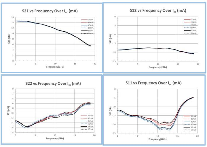
**Note:** The s-parameter gain results shown above were performed using a test fixture.
