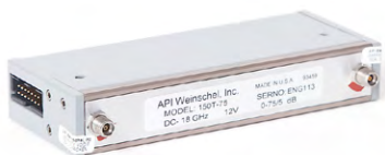
Model 150 Relay Switched Programmable Attenuator 50 ohm Bidirectional Unit operating DC to 18 GHz frequency range.
