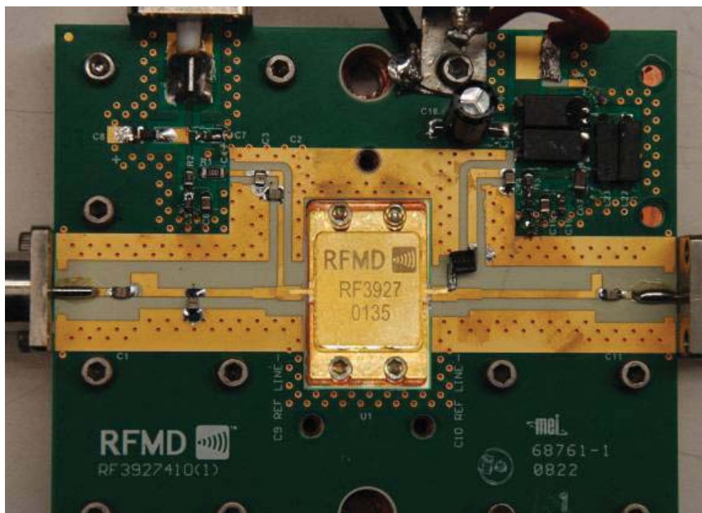
Figure 3. Compact S-Band GaN HPA
