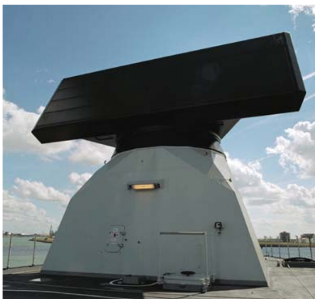
Figure 1. Long Range Surveillance L-Band Phase Array Radar
