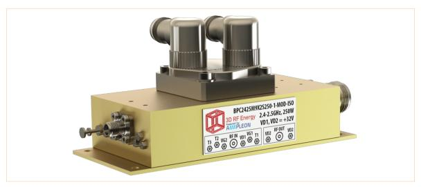
The BPC2425M9X2S250-1-MOD-ISO is a compact 250W, 2.45GHz power amplifier module designed for CW industrial applications. It integrates an Ampleon BPC2425M9X2S250-1 production pallet with a robust housing, filtering, internal isolator, and RF connectors, making it suitable for system integration as well as pallet evaluation.
