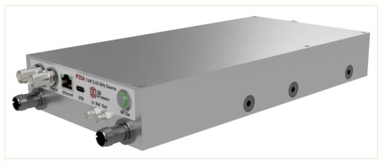
The P25A is a compact 1kW, 2.45GHz RF power source designed for industrial applications. It integrates two 500W production pallets with a MMIC driver, robust housing, internal isolator, and an RF exciter.
