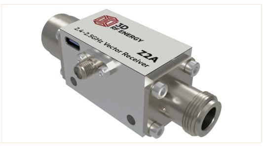
Vector receiver technology is a key component of all of 3D RF Energy's microwave energy systems, where it is used to perform high-accuracy real-time measurements of load impedance, delivered power, and output phase.
