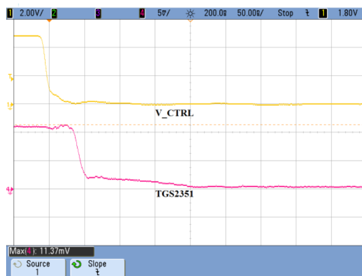
Fig. 4 FET based driver circuit (Fig. 3) turns GaN Switching TGS2351 on and Off within 50 nS.
